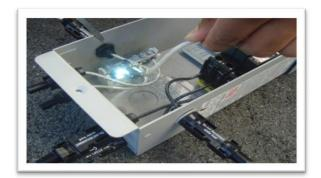
Figure 18 – Actual Arc Fault
