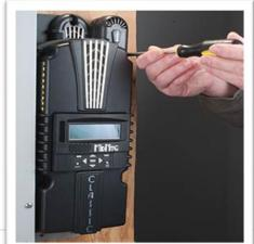
Remove the four screws holding the front cover of the Classic charge controller (see Figure 27).
