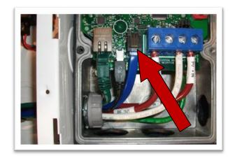
Figure 105 - Battery Temperature Sensor
