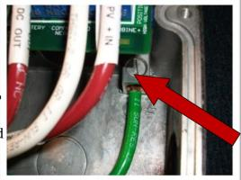
Figure 10 - Chassis Ground Point
